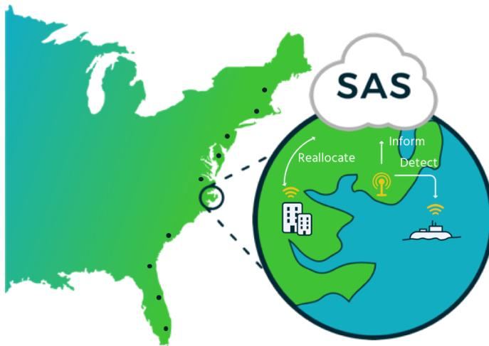
There will also be Environmental Sensing Capability (ESC) operators. The ESCs will consist of networks of sensors that will detect the presence of signals from federal systems in the band and communicate that information to one or more SASs to facilitate protection of federal operations in the band. The ESCs will also protect incumbent users within a
